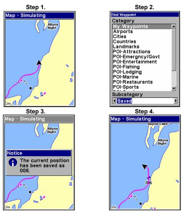
Sequence for setting a waypoint. Step 1: while traveling, *quickly* press WPT *twice* to call up Find Waypoint screen (seen in Step 2) and set a point. Step 3: message says the waypoint has been saved. Step 4: vehicle continues on its way; number waypoint symbol is visible on map.
